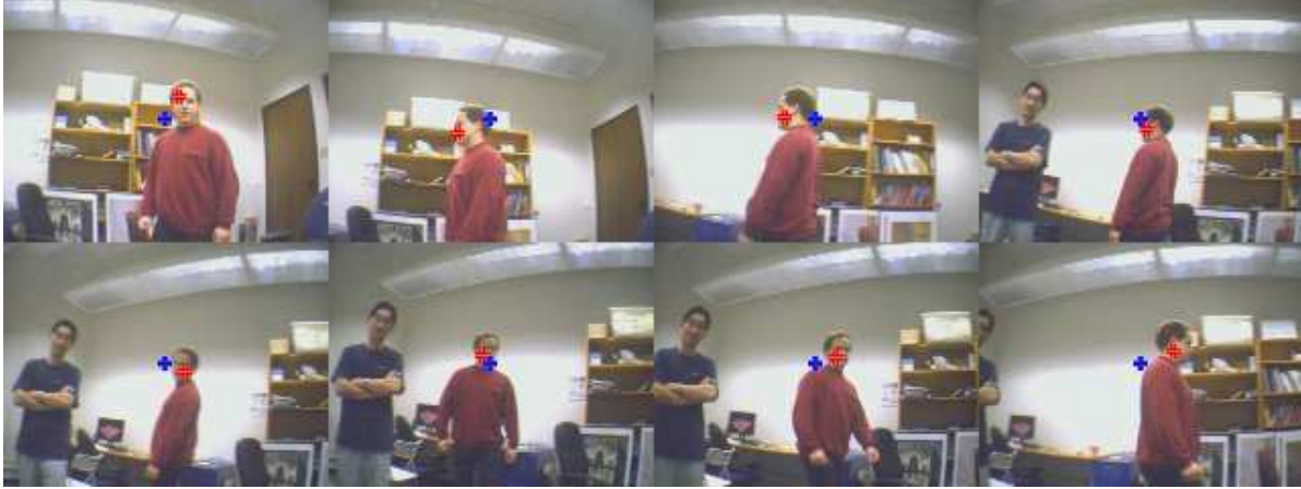
Figure 8: Sequence of images (top left to bottom right) of tracking a face. The red crosses indicate the estimated target position. The dark blue crosses mark the center of the image.
