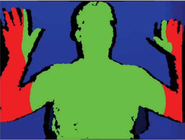
Fig. 8: Output of the user posture analysis system. The body parts which are outside of the safety volume are marked in red.
