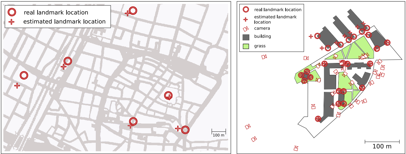
Fig. 3. True and estimated landmark locations in Freiburg downtown overlaid on a street map (left) as well as for the Freiburg campus experiment overlaid on a building plan (right). Note that due to copyright reasons, we do not visualize the results using the original satellite images.
