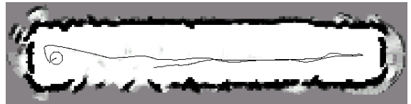
Fig. 6. This image depicts an occupancy grid map obtained with scan counting ( n = 1 ).
