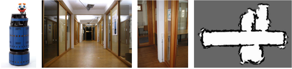
Fig. 4. The right image depicts the B21r robot Albert used to carry out the experiments. Albert is equipped with a SICK PLS laser range sensor and 24 ultrasound sensors. Both images in the middle show photographs taken within the corridor of our office environment. The right image depicts a coverage map learned by Albert using its ultrasound sensors in this environment.
