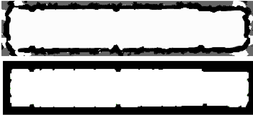
Figure 3.4: The top image depicts a coverage map learned from ultrasound data using our sensor model and map update technique. In this experiment, most of the obstacles fit into the grid discretization and therefore only a few cells show partly occupied cells. The lower image illustrates the corresponding ground truth map learned from laser range data.
