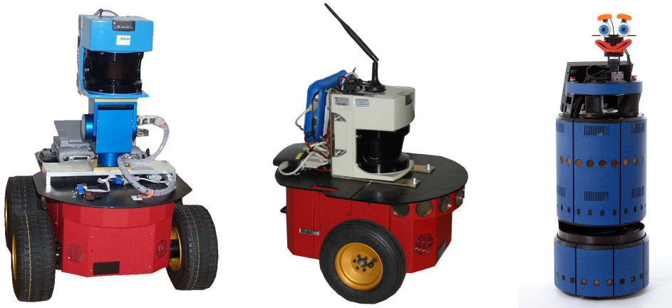
Figure 6.4: Different types of robot used to acquire real robot data used for mapping (ActivMedia Pioneer 2 AT, Pioneer 2 DX-8, and an iRobot B21r).
