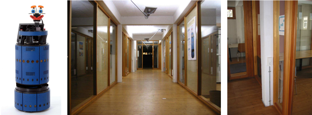
Figure 3.5: The left image depicts the B21r robot Albert used to carry out the experiments. Albert is equipped with ring of 24 ultrasound sensors. The other images show photographs taken within the corridor of our office environment.
