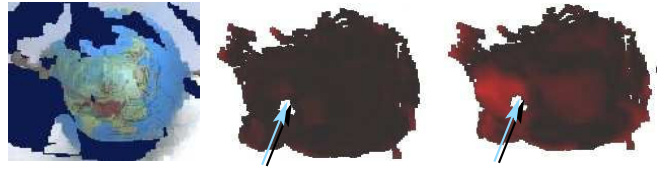
Fig. 4. Left: Color 3D point cloud of the surface of a ball. Middle: Error mask showing the differences between the simulated deformations and the observed deformations of a good parameter estimate (our approach). Red pixels indicate high errors and dark pixels indicate low errors. Right: Error mask for suboptimal parameters where the observed deformation is not in line with the prediction one (red area). The hole in the model (arrow) results from occlusions due to the physical interactions of the manipulator with the object.
