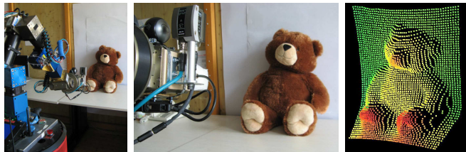
Fig. 1. Reconstructing a model of a deformable object: manipulation robot (left) equipped with a depth camera and force-feedback sensor (middle) and the 3D perception of the robot (right).
