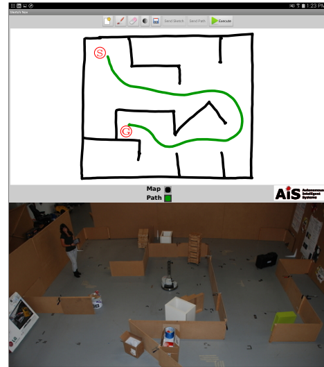
Fig. 1. Top: Snapshot of the tablet interface. Figure shows the drawn map and the path (green). The starting (S) and goal (G) positions are annotated. Bottom: The environment used for the experiments.
