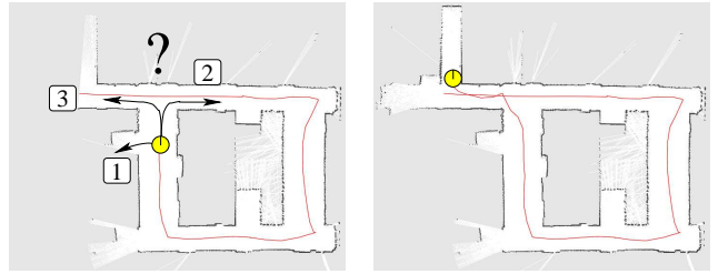
Fig. 1. Suppose the robot has a high pose uncertainty and has to decide where to go next. Shown are three opportunities in the left image. Our map and pose entropy-driven exploration system chooses action 3 (as depicted in the right image) since it provides the highest expected utility (see also Figure 7).
