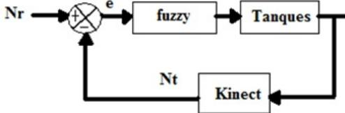
Figure 7. Block diagram of the control loop
