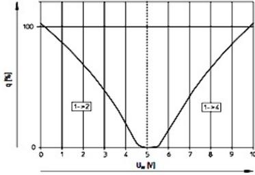
Figure 6. V-Q diagram of the proportional valves
