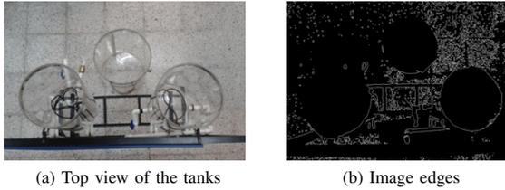
Figure 2. Processing results over the top view image
