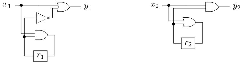
Consider the sequential hardware circuits above. The initial values of the registers are  $r_1 = 0$  and  $r_2 = 0$ . In Exercise Sheet 1 you already constructed the transition system  $T_1$  for the hardware circuit on the left.
