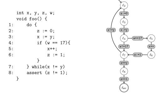
Give two error traces  $\pi_1$ ,  $\pi_2$  and construct corresponding interpolant automata  $\mathcal{A}_1, \mathcal{A}_2$ such that the inclusion  $\mathcal{L}(\mathcal{A}_{\mathcal{P}}) \subseteq \mathcal{L}(\mathcal{A}_1) \cup \mathcal{L}(\mathcal{A}_2)$  holds.
