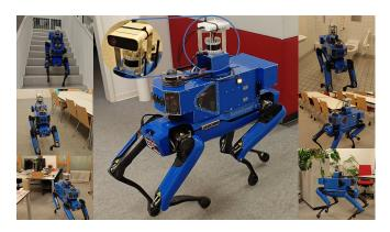
Fig. S.6. Boston Dynamics *Spot* robot traversing a two-story office building with multiple types of rooms. The quadruped is equipped with an Azure Kinect RGB-D camera and a 3D LiDAR. We obtain accurate pose estimates from LiDAR-based odometry estimation.
