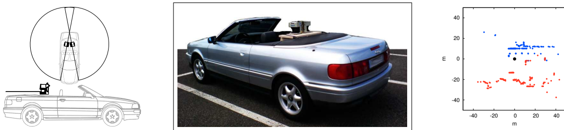
Fig. 5. Left: arrangement of two SICK laser range finders on a convertible (middle) used for gathering real data. Each laser has a field of view of 180 degrees and can detect objects as far as 80 meters with an angular resolution of 1 degree at 75Hz. The arrangement of the two lasers provided a 340 degree field of view (right).
