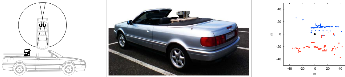
Fig. 6. Left: arrangement of two SICK laser range finders on a convertible (middle) used for gathering real data. Each laser has a field of view of 180 degrees and can detect objects as far as 80 meters with an angular resolution of 1 degree at 75Hz. The arrangement of the two lasers provided a 340 degree field of view (right).
