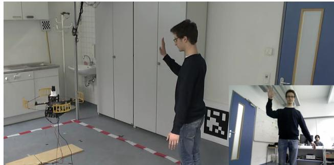
Fig. 1. Our approach enables a quadcopter to follow a person and to understand simple gesture commands such as “follow me”, “take picture”, and “land”.
