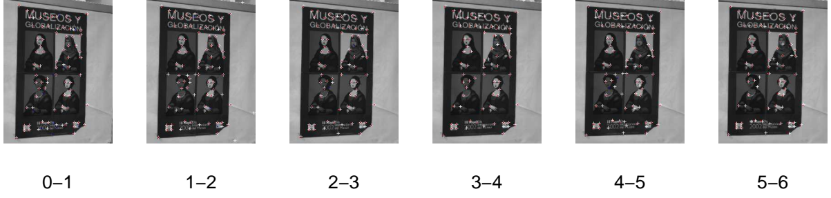
Figure 1: Sequence of images with persistent points (red), lost points (blue) and points detected (white).
