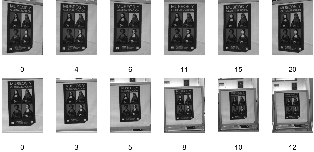
Figure 3: The top sequence shows images of a poster from different viewpoints. The bottom sequence shows the same poster with changes in scale.
