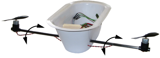
Fig. 2. This image shows the gondola with two rotors for pitch and thrust control. They can be rotated by 180 degrees.
