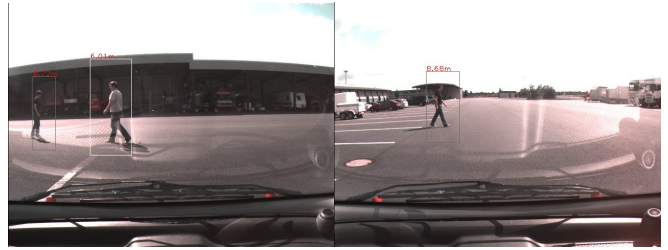
Fig. 4. Two images from parking lot dataset. Brighter rectangles indicate a high detection probability. On the left: the far away pedestrian receive a smaller vote with respect to the foreground person. On the right: a classic pedestrian crossing in simulated. Pedestrian distances are written in red.
