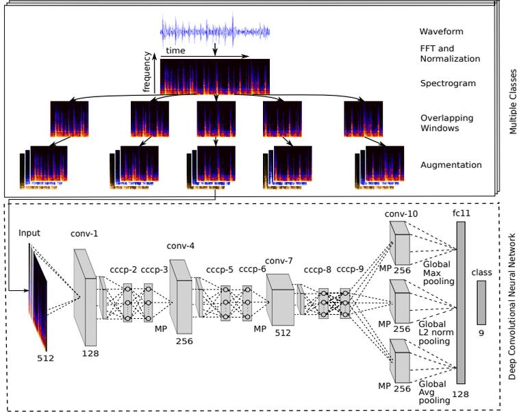
**Fig. 1** Overview of our terrain classification pipeline. Raw audio signal of the terrain interaction is first transformed into its spectrogram representation and then piped into a DCNN for feature learning and classification. MP refers to max pooling.
