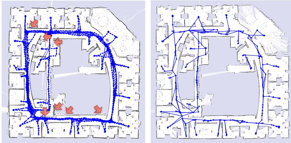
**Figure 8:** Map and pose graph obtained when mapping the Intel Research Lab. Left: Standard approach, 1802 laser scans, 3916 edges. Right: Our approach preserves the sparsity of the pose graph, 250 laser scans, 349 edges. Arrows indicate locally blurred areas or small alignment errors in the map obtained by the standard approach. In contrast to our approximate marginalization technique, exact marginalization would result in 13052 edges.
