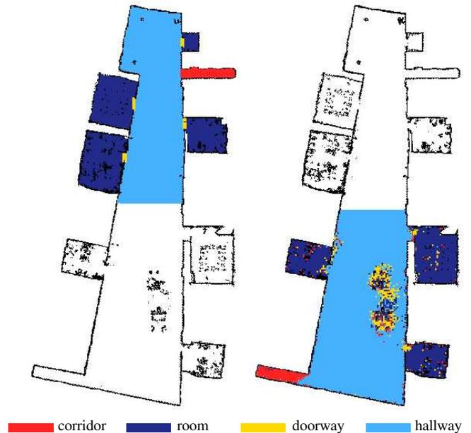
Fig. 6. The left image show the training data used to train the classifiers and the right image the classification results of our sequential AdaBoost classifier.
