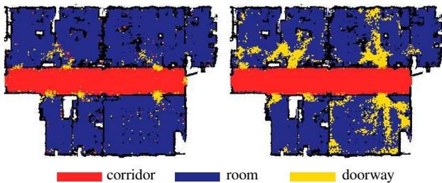
Fig. 9. The left image show the classified test data of our sequential AdaBoost algorithm in building 79. The right image depicts the result obtained with AdaBoost.M2. As can be seen, the error of AdaBoost.M2 is much higher compared to our approach.
