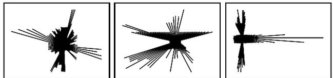
Fig. 2. Example scans recorded in a room, a doorway, and a corridor.
