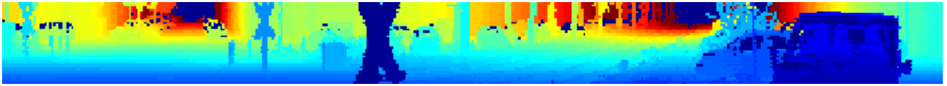
Fig. 2. A depth image built from a single rotation of a Velodyne scan
