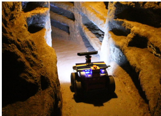
Fig. 1. Remotely operated robot in an underground catacomb. The robot streams Kinect depth data for building a map to a remote operator.
