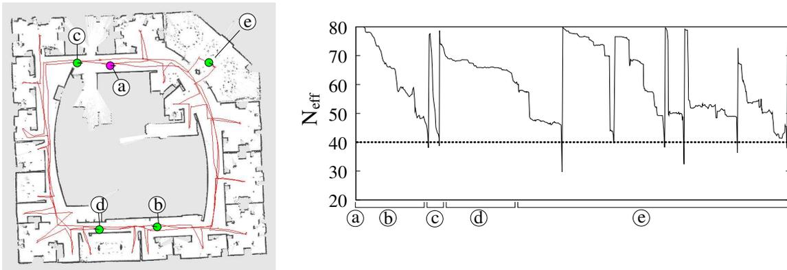
Figure 7. The left image depicts a map of the Intel Research Lab as well as the trajectory of the robot during data acquisition. The robots started at (a), traversed the big loop (b), and closed it (c). It then re-visited the loop again (d) and started exploring the rooms (e). The right plot shows the evolution of  $N_{eff}$ . Each time it drops below 40 a resampling is performed.
