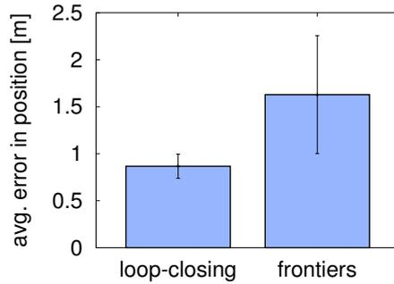
Figure 9. Comparison of our loop-closing strategy with a purely frontier-based exploration technique. The left bar in this graph plots the average error in the pose of the robot obtained with our loop-closing strategy. The right bar shows the average error obtained with a frontier-based approach. As can be seen, our technique significantly reduces the distances between the error in the relative pose estimates.
