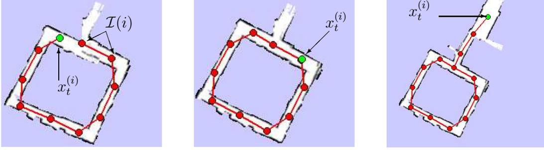
Figure 3. The (red) dots and lines in these three image represent the nodes and edges of  $\mathcal{G}^{(i)}$ . In the left image  $\mathcal{I}(i)$  contains two nodes. In the middle image the robot is closing a loop. Afterwards the robot continues exploring unknown terrain (right image).
