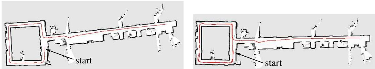
*Figure 1. Two different maps obtained from a real world experiment performed in Sieg Hall at the University of Washington. In the left image the robot traversed the loop on the left side only once before it entered the corridor. Accordingly, it was unable to localize itself correctly when it closed the loop. In the right image, the robot traversed the loop twice and therefore could correctly estimate its position in the map. The accuracy of the resulting map therefore is much higher.*
