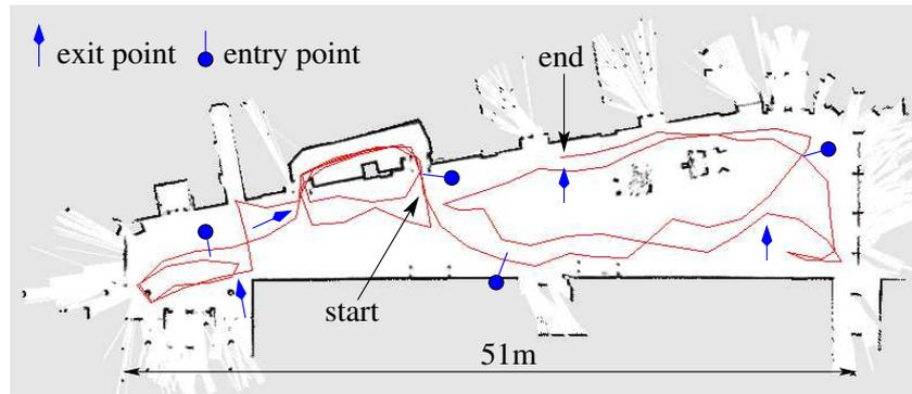
Figure 8. This image shows the resulting map of an exploration experiment carried out using a Pioneer 2 robot equipped with a laser range scanner in the entrance hall of the Department for Computer Science at the University of Freiburg. Also shown is the path of the robot as well as entry and exit points where the robot started and stopped the active loop-closing process.
