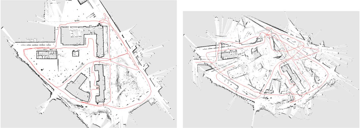
Figure 6. The campus of the Department of Computer Science at the University of Freiburg. The left image shows a map created with the improved Rao-Blackwellized mapping technique, whereas the right image was constructed with a Rao-Blackwellized mapper lacking the improved techniques introduced in this paper.
