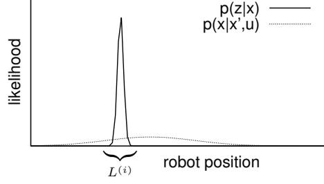
Figure 2. The two components of the motion model. Within in interval  $L^{(i)}$  the product of both functions is dominated by the observation likelihood. Accordingly the model of the odometry error can safely be approximated by a constant value.
