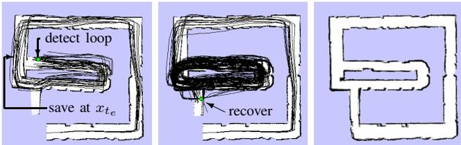
Fig. 3. This figure shows the same experiment as depicted in Figure 1, but using our recovering technique. In the left image the robots saves the set of approximated particles at time step  $t_e$  and later on recovers the vanished hypotheses (middle image). This allows the robot to correctly close the outer loop (right image).
