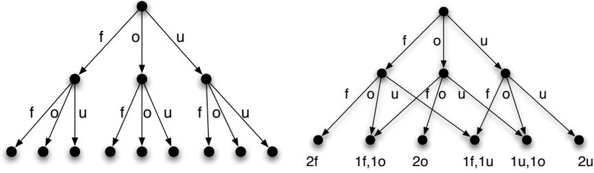
**Fig. 2:** Left: all combination of measurement combinations that can occur for  $n$  beams, here with  $n = 2$ . In the figure, f=free, o=occupied, and u=unknown. The number of combinations is  $3^n$ . Right: Since the order of the measurements is irrelevant, the number of *possible outcomes* is quadratic in  $n$ .
