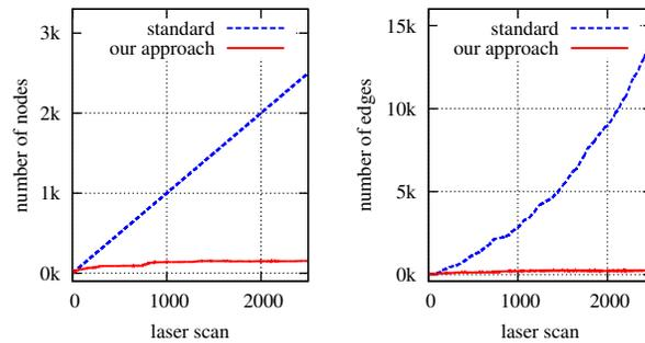
**Fig. 8:** Results of an experiment in which the robot moved around in an office environment for an extended period of time. In this experiment, our algorithm discarded all laser scans whose expected information gain was below a threshold.
