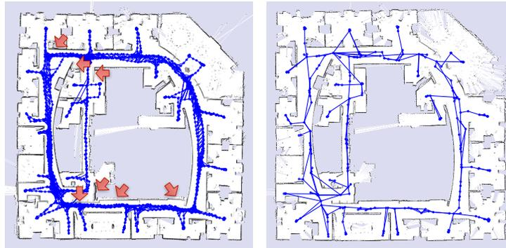
**Fig. 5:** Intel Research Lab. Left: Standard approach, 1802 laser scans, 3916 edges. Right: Our approach preserves the sparsity of the pose graph, 250 laser scans, 349 edges. Arrows indicate locally blurred areas or small alignment errors in the map obtained by the standard approach. In contrast to that, exact marginalization would result in 250 laser scans as well, but in 13052 edges.
