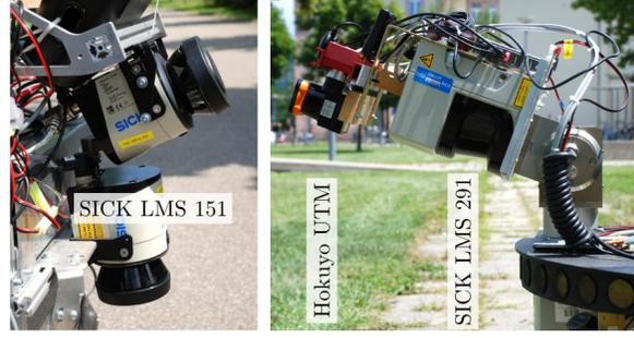
Figure 6: Sensors used in the evaluation.
