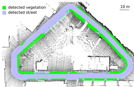
Figure 13: Mapping a large outdoor environment. The laser was tilted at a fixed angle of 20 degrees while the robot was moving. The figure shows a 2D projection of the 3D map.
