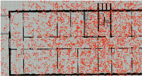
(a) Particle filter initialization using a uniform distribution.
