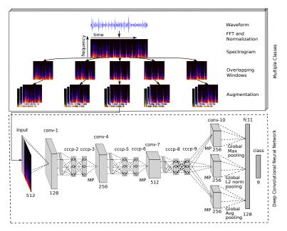
**Fig. 1** Overview of our terrain classification pipeline. Raw audio signal of the terrain interaction is first transformed into its spectrogam representation and then piped into a DCNN for feature learning and classification. MP refers to max pooling.
