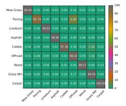
**Fig. 8** Confusion matrix for classification runs using data from a mobile phone microphone. Paving and Cobble show decreased performance due to false positives with Offroad and Grass.
