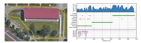
**Fig. 7** The map on the left shows the trajectory taken by the robot during a classification test run using a mobile phone microphone. The variation in speed along the path is indicated in red and wider red points denote slower speed. The graph on the right shows the classification result, along with the corresponding probabilities for the path shown in the map. True positives are shown as green markers and false positives are shown are red markers.
